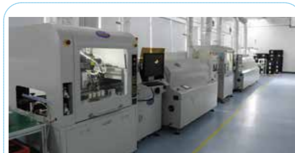
Note: The automatic spraying line of three-proofing lacquer
